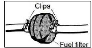
Empty the fuel tank by disconnecting the tube situated at the inlet of the fuel filter and follow the instructions in the engine manual. Ensure there is no potential for ignition sparks before proceeding. Proceed with caution.
