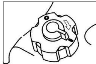
**IMPORTANT** The choke must be opened as soon as the engine is running smoothly. Using it when the engine is already warm can foul the spark plugs and cause the engine to run erratically.
