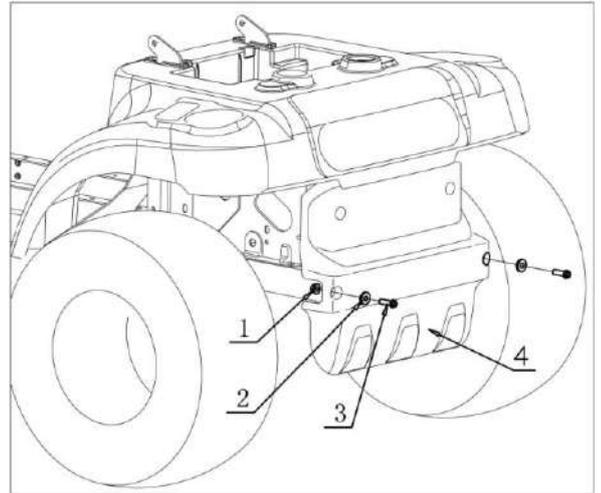
b. Insert the bushing (2) into the two holes where the bolts were just removed, align the towing plate (5),
