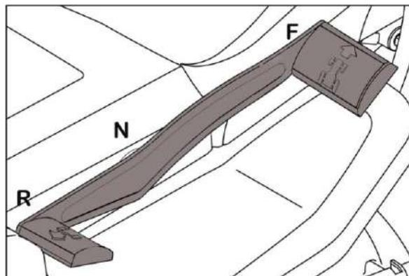
Reverse is engaged by pressing the pedal with the heel towards «R».
